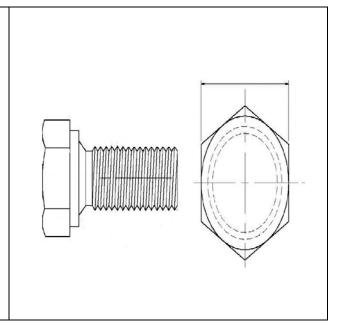
**Plug Size:** 3/4"-16 UNF, 7/8"-14 UNF, 1-1/8"-12 UNF, 1-1/2"-12 UNF, 1-3/4"-12 UNF, 1-5/8"-12 UNF, 2"-12UNF (We also manufacture this Plug as per Customer Drawing / Dimensions)
